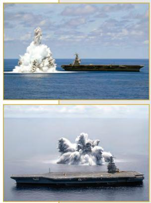
Full Ship Shock Trials (FSST) is a series of, in our case, three blasts experienced over the course of about two months. The blasts start a few hundred yards from the ship and progress closer with each one, testing the ability of each new ship design to respond to battle damage.
